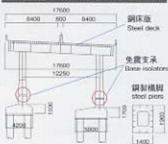
復旧後断面 Cross-section after the restoration
